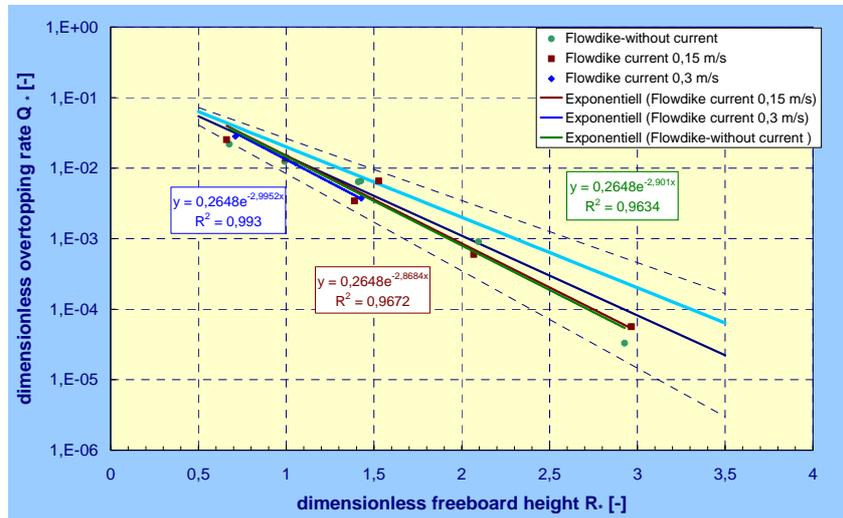
Fig. 7. Wave overtopping data influenced by current (non-breaking)
