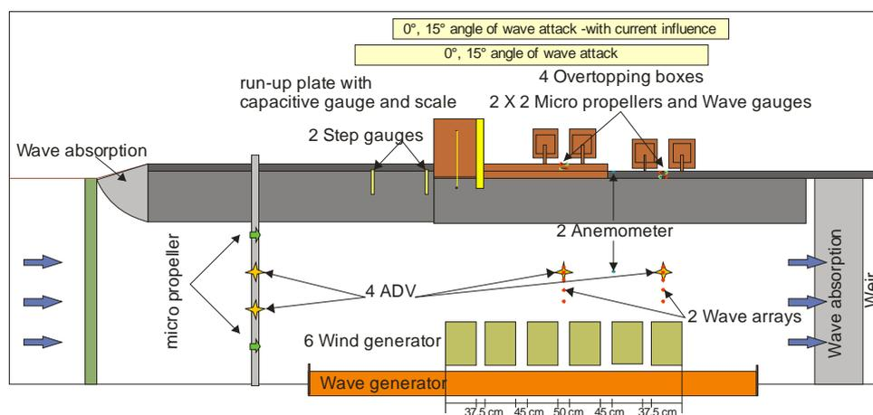
**Fig. 1. Overview of the model with instruments and flow direction**
