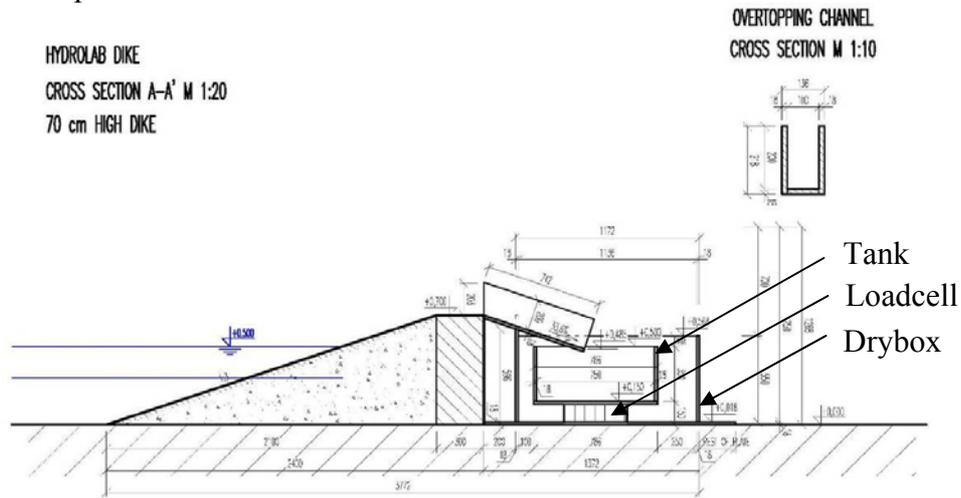
**Fig. 2. Cross section of overtopping unit for the 70cm crest**
