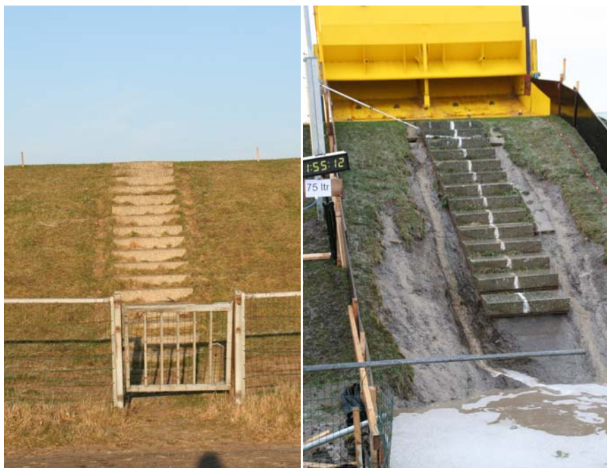
Figure 20. Afsluitdijk. Staircase with fence, before and after testing, section 3.
