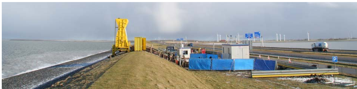
Figure 3. Set-up of Wave Overtopping Simulator close to a highway (February 2009)
