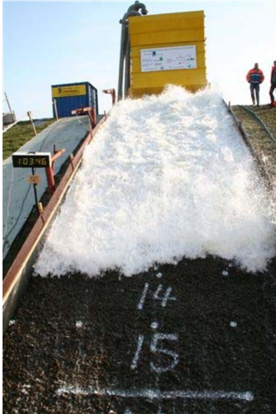
Figure 16. Kattendijke, Zeeland. Final test on elastocoast, section 3.
