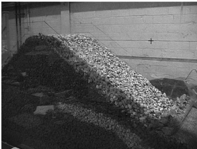
Fig. 4. The model filter layer and core before armour placement.
