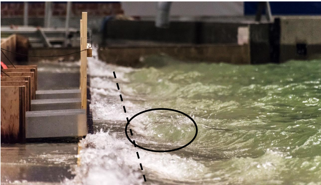
Fig. 7. Wave breaking on the lower slope
