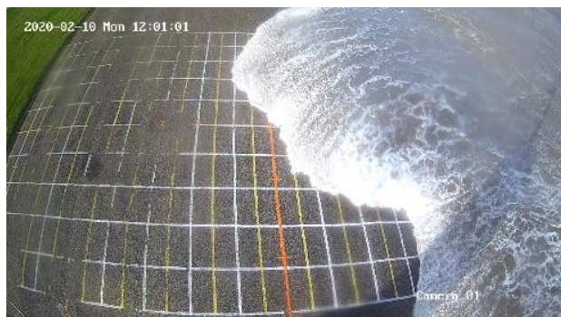
Figure 3 - Snapshot of a very oblique wave running up the slope during storm Ciara.
