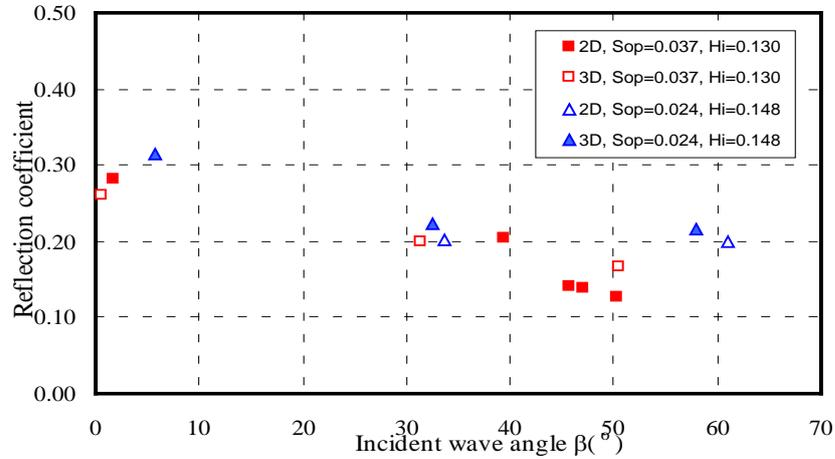
Figure 3 Comparison of long-crested and short-crested waves for smooth structures
