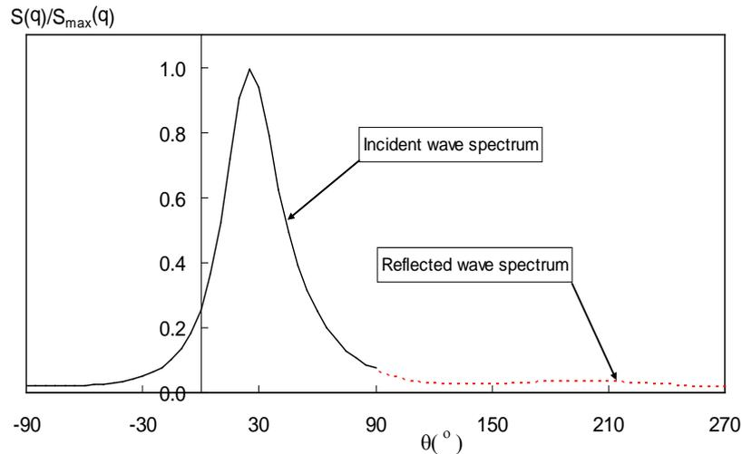
Figure 8 Incident and reflected wave spectra in spatial domain
