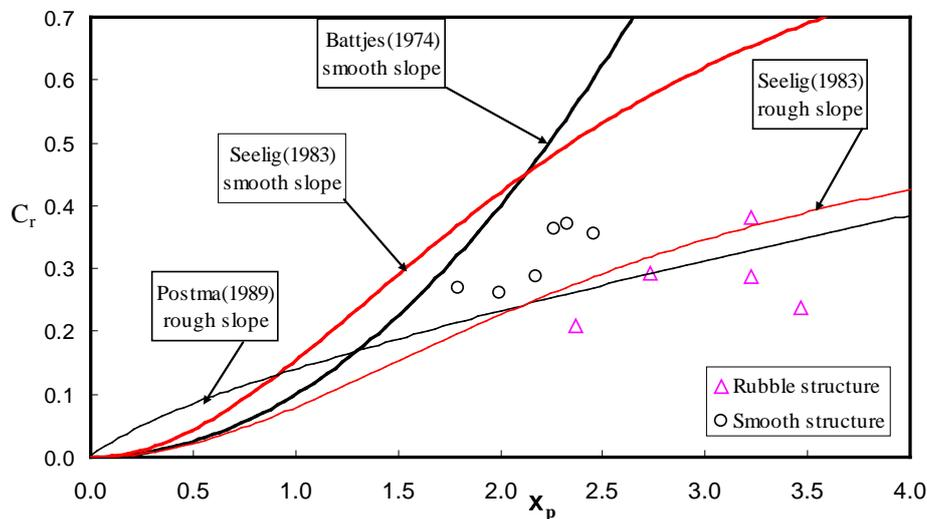
Figure 4 Comparisons of the measurements and predictions
