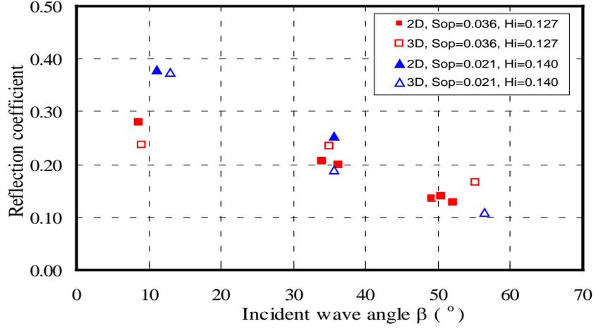
Figure 2 Comparison of long-crested and short-crested waves for rubble mound structures
