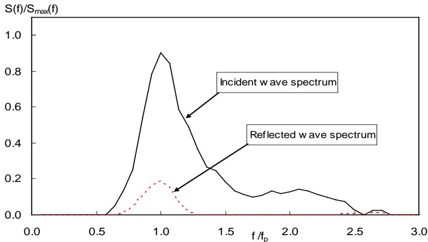
Figure 7 Incident and reflected wave spectra in frequency domain
