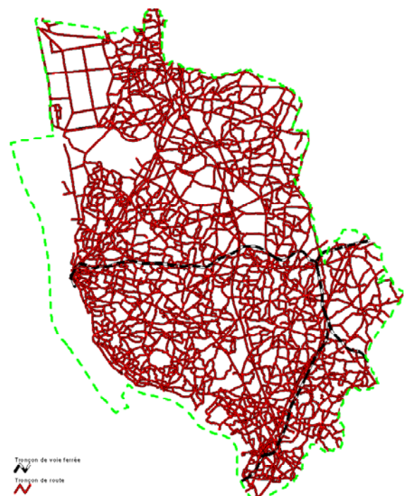
Figure 9. Roads and railways used in calculation of flood damage in the Haute Gironde
