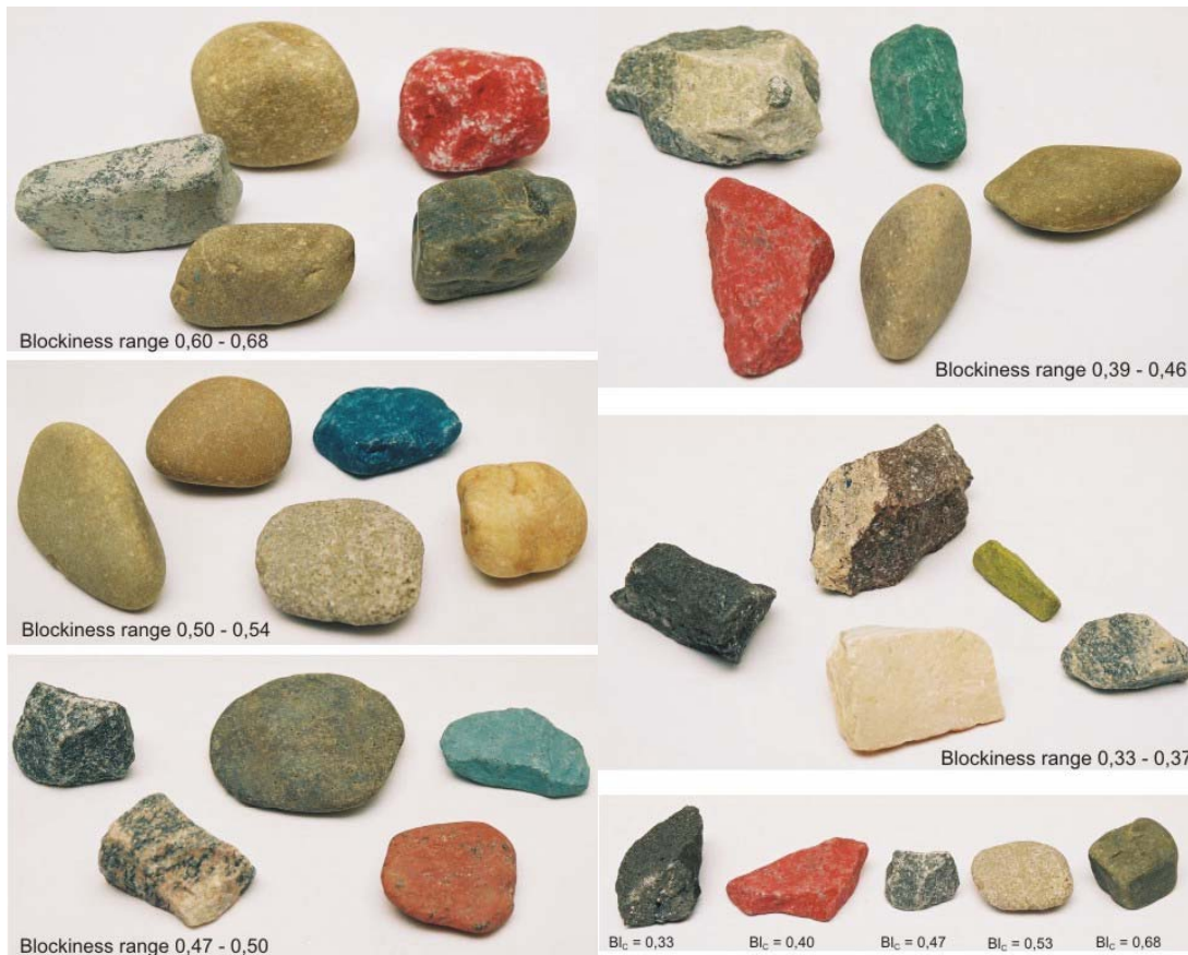
Figure 6. Groups of rocks in various ranges of the blockiness coefficient
