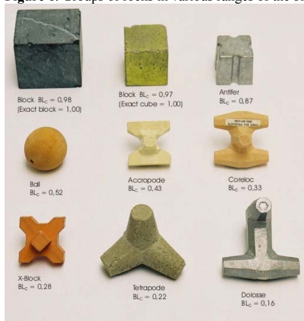
Figure 7. Blockiness coefficients for armour units
