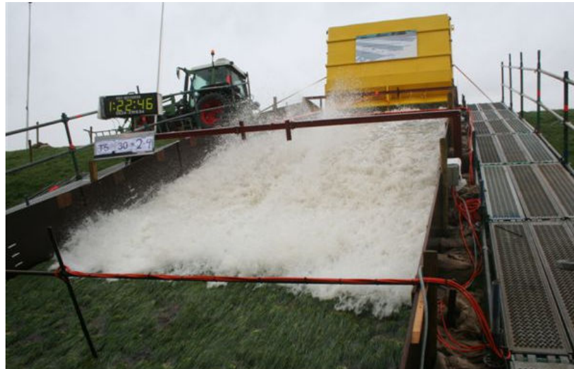
Figure 7: Overtopping simulator discharging a large volume on the inner slope of a dike
