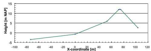
Figure 3. Schematized cross-section of the sea dike in the case study.
