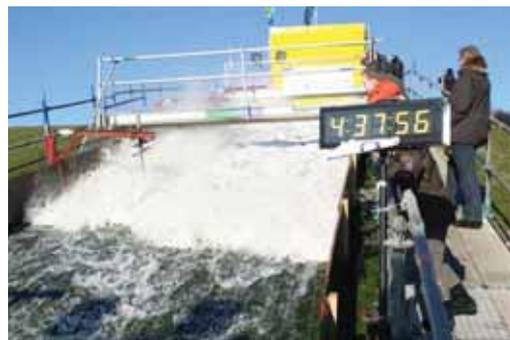
Figure 6. The wave overtopping simulator releases 22 m<sup>3</sup> of water over 4 m width in about 5 s. It simulates a large overtopping wave with an average discharge of 75 l/s per m.
