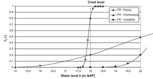
Figure 2. Fragility curves for three failure mechanisms as function of the water level. Situation of high river discharge.
