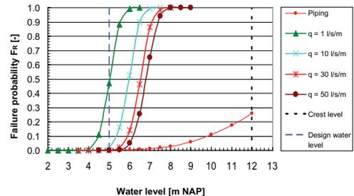
Figure 4. Fragility curves for piping and overtopping.
