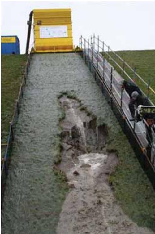
Figure 7. Damage to a dike section during a test with 75 l/s per m wave overtopping.
