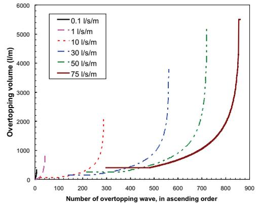
Figure 6. Overtopping distributions for various mean discharges.
