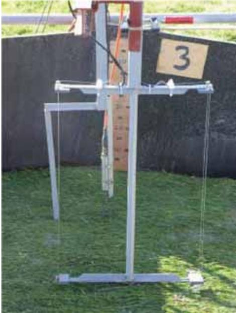
Figure 9. Flow depth instrument.
