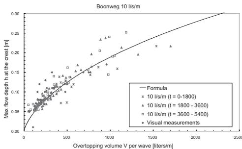
Figure 10. Flow depth measurements.
