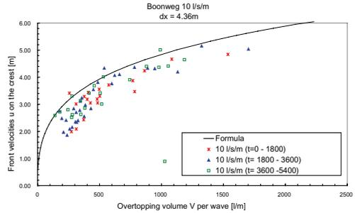
Figure 11. Calculated front velocities between to sets of instruments.
