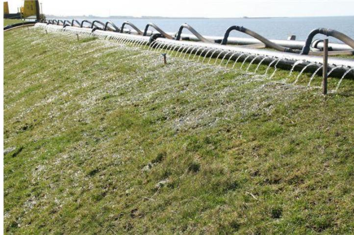
**Figure 1. Overflow test on a sea dike over a length of 30 m during 56 hours to induce sliding.**
