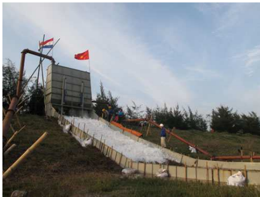
Figure 1. Wave overtopping simulator.
