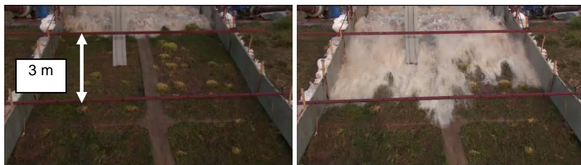
Figure 3. Movement of the front of a wave over 3 m within 0.8 s, giving a front velocity of 3.75 m/s.
