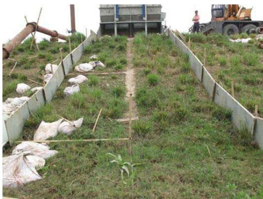
Figure 2. Test point TT_03, mixture of Bermuda and Vetiver grass.
