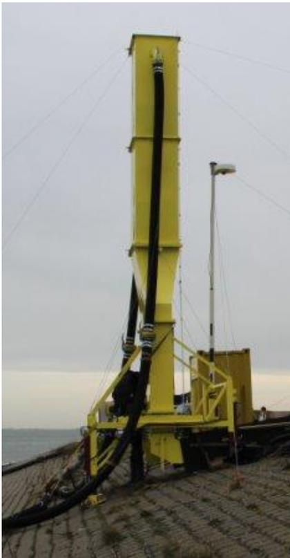
**Figure 4. Wave Run-up Simulator seen from the side.**
