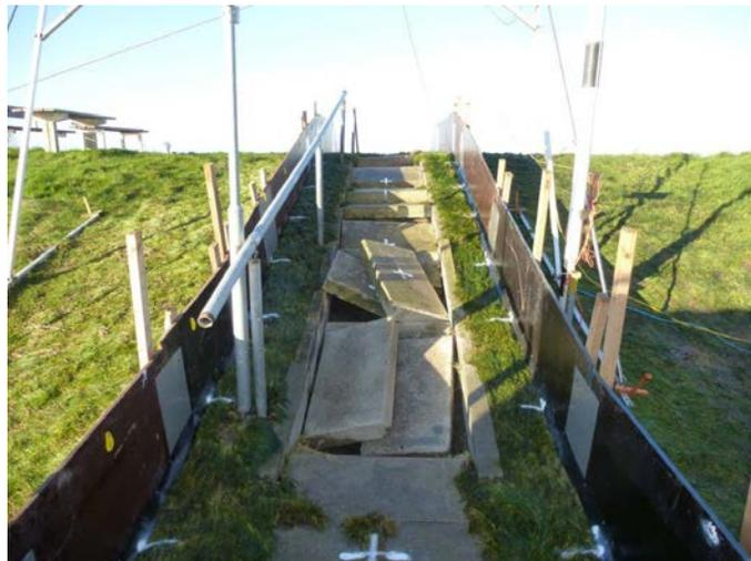
**Figure 7. Testing a staircase with wave run-up simulation.**
