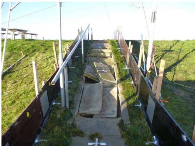
Figure 9. Testing a staircase with wave run-up simulation.
