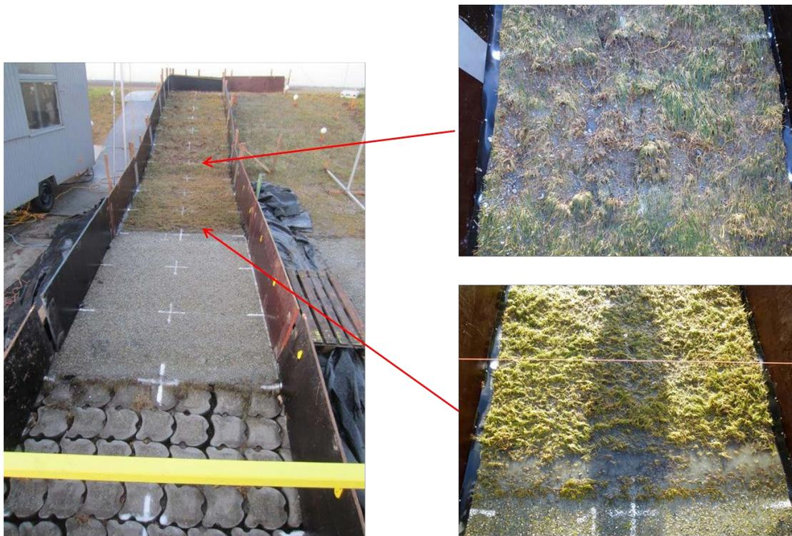
Figure 10. Damage to the transitions after test 1, showing hardly damage to initial damage
