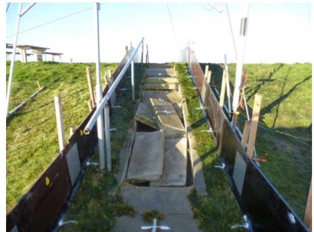
Figure 12. Testing a stair case with the new Wave Run-up Simulator in 2014.
