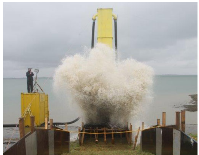
Figure 17. Measuring impacts by overtopping waves on a quay area towards a vertical step of a stair case type structure.
