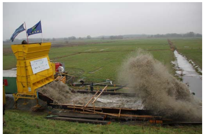
Figure 16. Measuring impacts by overtopping waves on a promenade towards a vertical storm wall.
