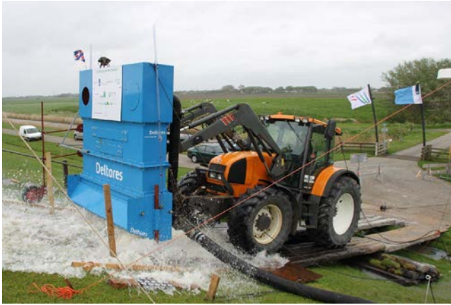
Figure 7. Test with Wave Impact Generator.
