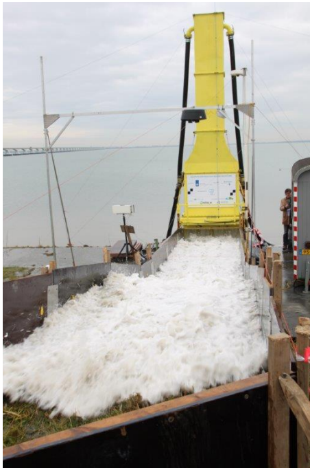
Figure 11. The new Wave Run-up Simulator, designed in 2013.
