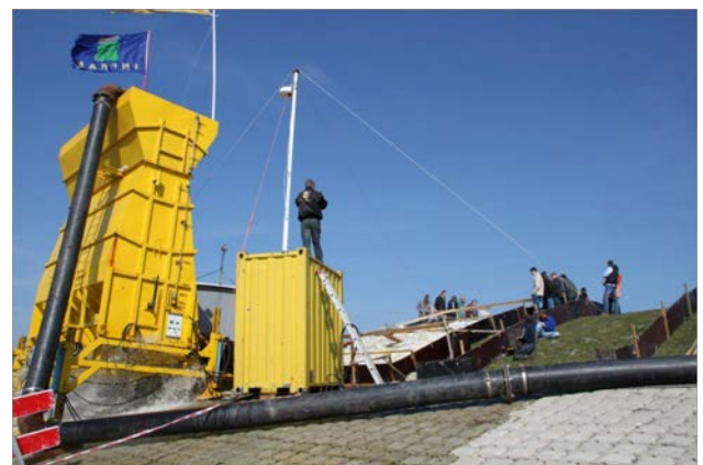
Figure 9. Set-up of the pilot wave run-up test at Tholen, using the existing Wave Overtopping Simulator.
