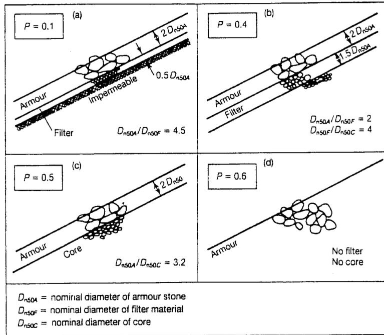
Figure 2 Notional permeability factor P for various structures
