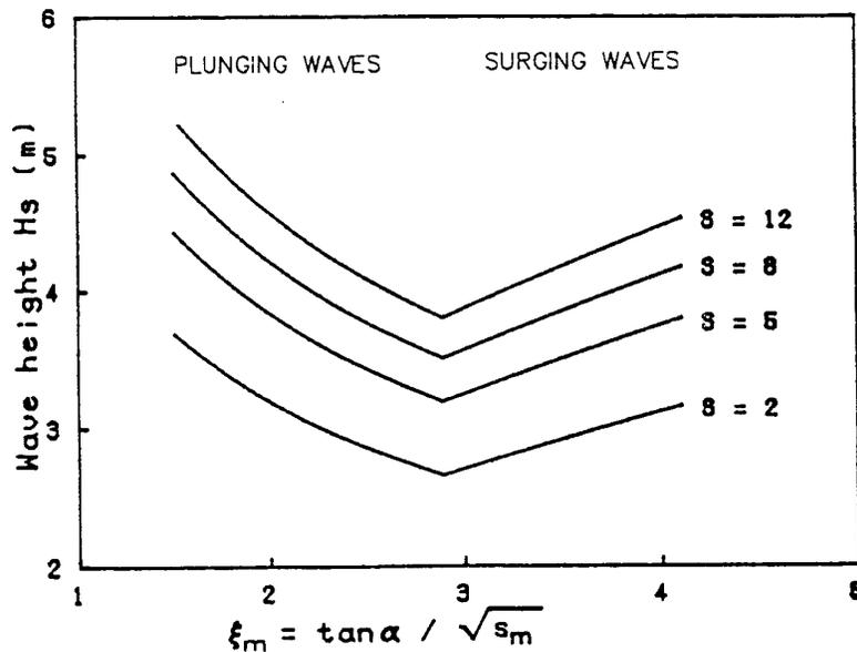
Figure 3 Wave height versus breaker parameter; influence of damage level
