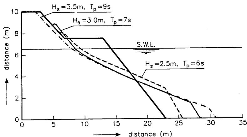
Figure 16 Example of influence of wave climate on a berm breakwater profile
