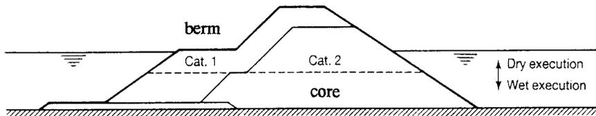
Figure 14 Cross-section of a berm breakwater
