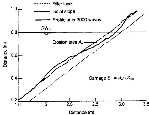
Figure 1 Damage S based on erosion area  $A_e$
