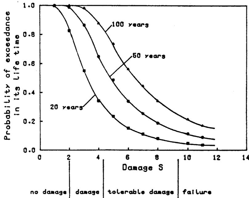
Figure 8 Probability of exceedance of the damage level  $S$  in the lifetime of the structure
