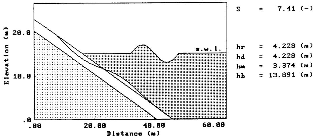
Figure 7 Calculated damage profile of a statically stable rock slope
