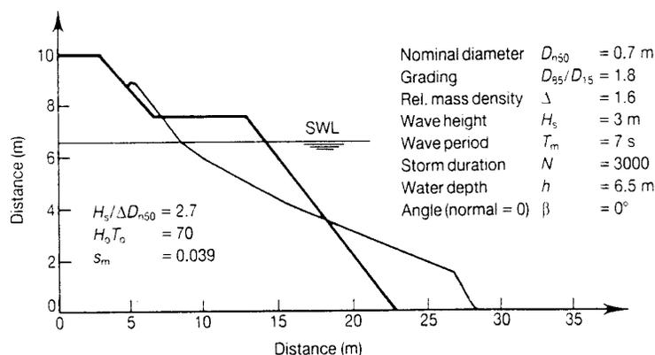
Fig. 15 Example of a computed profile for a berm breakwater
