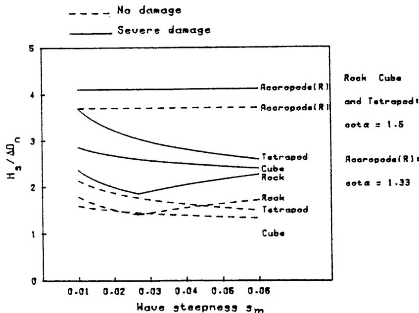
Figure 11 Comparison of stability of rock, cubes, tetrapods and accropode as a function of wave steepness
