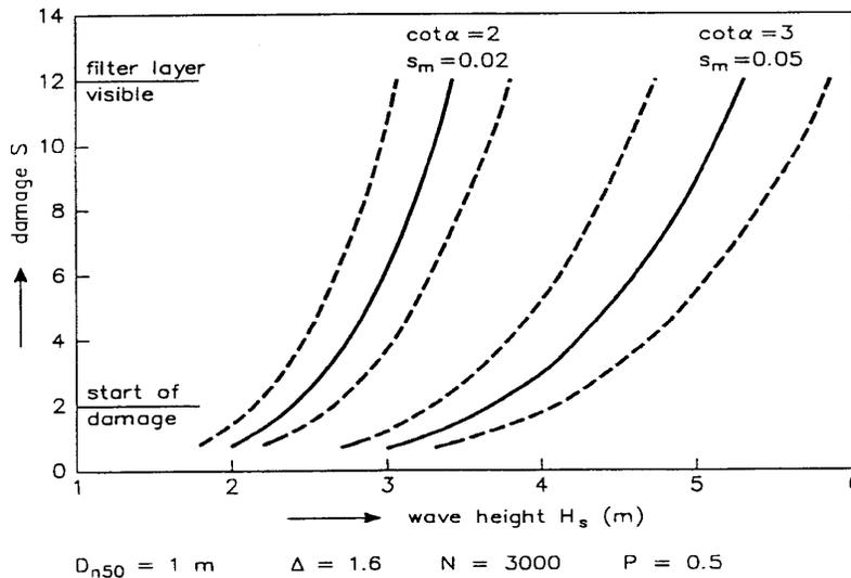
Figure 5 Wave height versus damage
