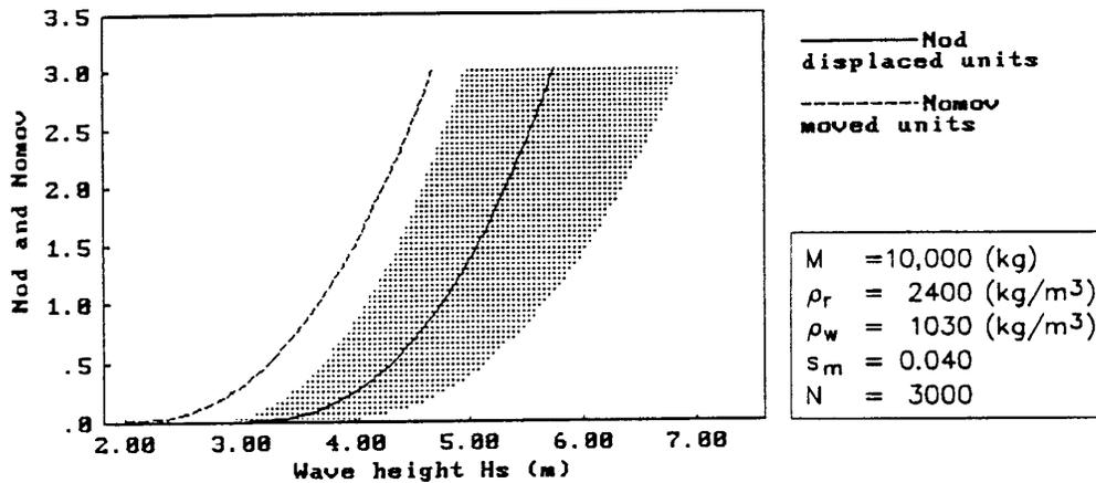
Figure 13 Wave height – damage curve for cubes with 90% confidence bands
