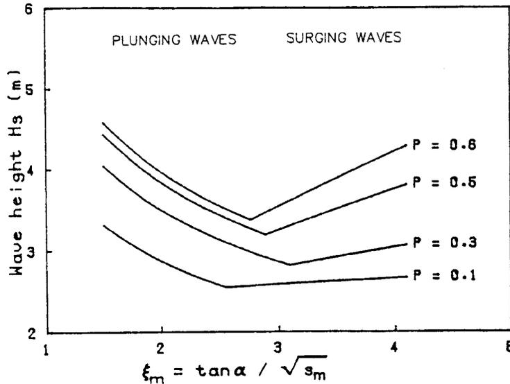
Figure 4 Wave height versus breaker parameter; influence of permeability
