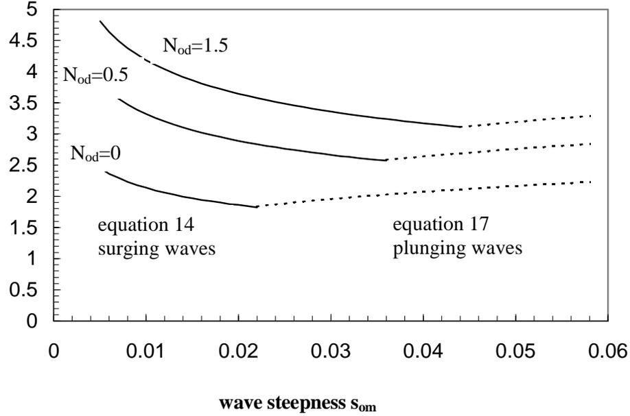
Figure 10 Stability number as a function of wave steepness for tetrapods with  $N=1000$
