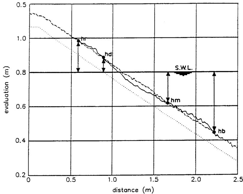
Figure 6 Damage profile (as measured) of a statically stable rock slope
