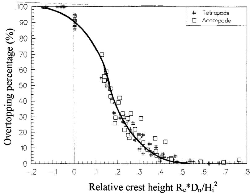
Figure 9 Percentage of overtopping waves as a function of crest height (conventional breakwater)
