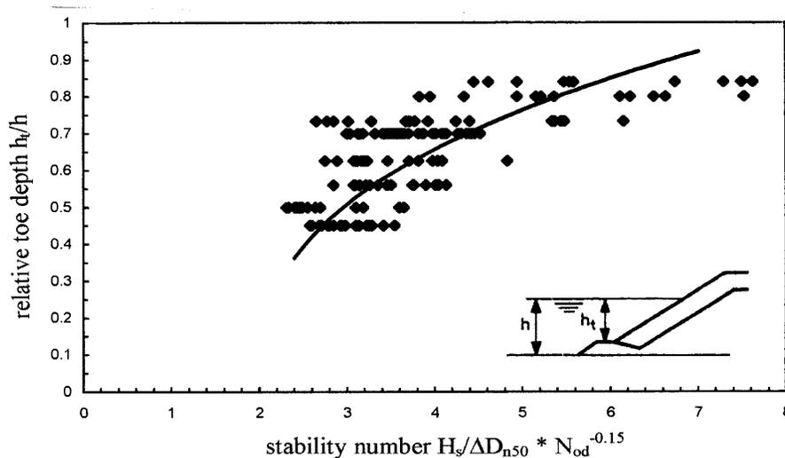
Figure 12 Toe stability as a function of relative depth  $h_t/h$  and damage level  $N_{od}$
