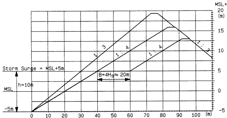
Figure 5 Example of different dike shapes and height with the same 2%-wave run-up level (from Pilarczyk, ed., 1990)
