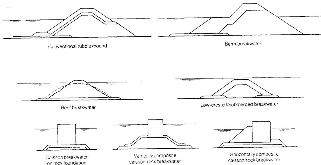
Figure 4 Basic breakwater concepts (from CUR/CIRIA, 1995)
