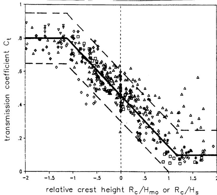
Figure 8 Simple relationship for wave transmission over rubble mound structures (van der Meer, 1993)
