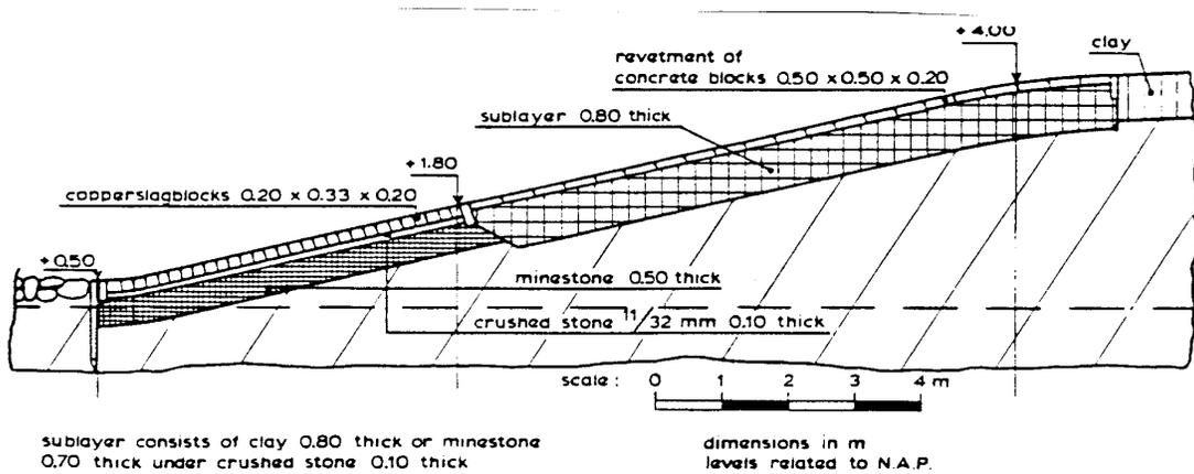
Figure 3 Example of dike protection (from Pilarczyk, ed., 1990)
