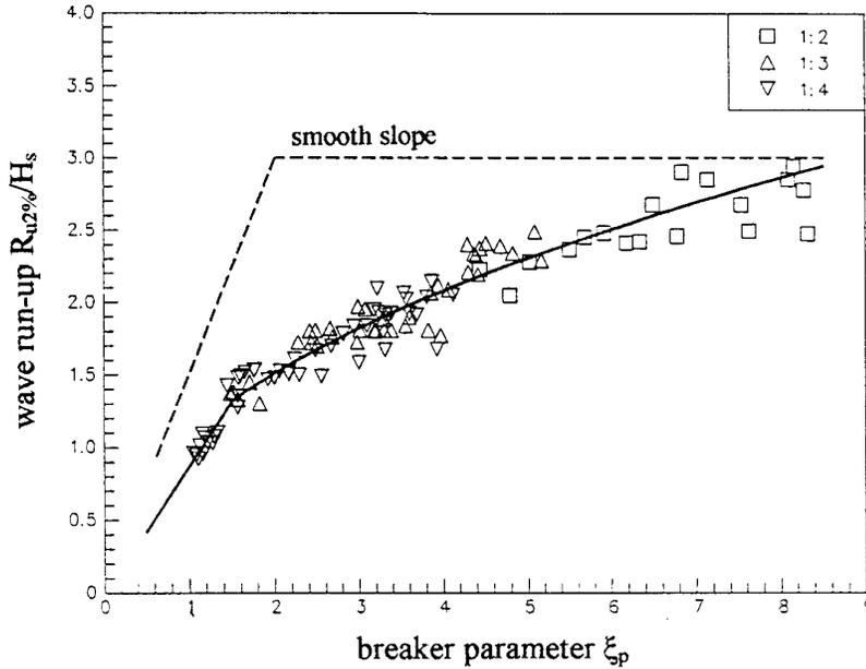
Figure 7 Wave run-up (2%) on rock slopes
