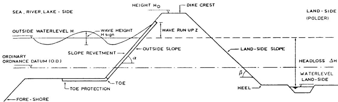
Figure 2 Schematisation of a dike (distorted scale)
