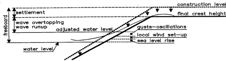
Figure 6 Important aspects when computing the dike height
