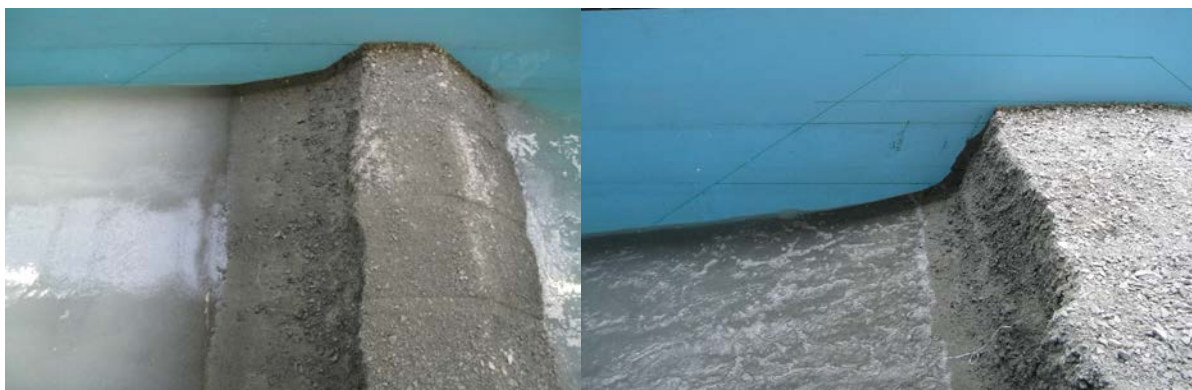
Figure 16 Photographs of Wide Grade bund after test D_SEA_150A (left) and after test E_SEA_200A (right).
