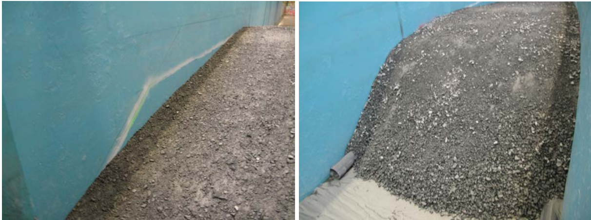
Figure 10. Front slope (left) and rear slope (right) after test C_SEA
