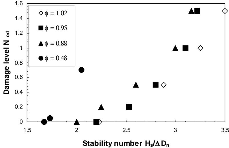
Figure 3 Stability of tetrapods for various packing densities
