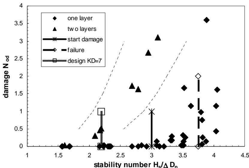
Figure 6 Stability of a single layer of cubes
