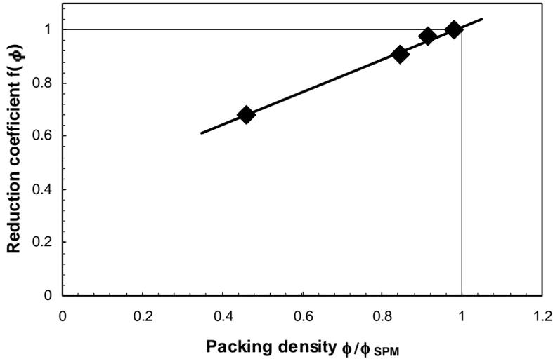
Figure 4 Influence of packing density on stability (of tetrapods)
