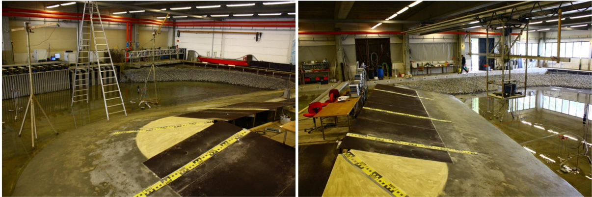
Figure 6: Model set-up with run-up boards and gauge scale at the P-dike (left) and at the N-dike (right).
