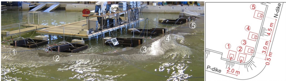
Figure 4: Numeration and position of overtopping units.
