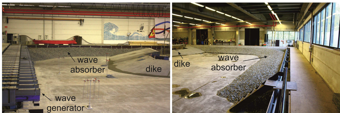
Figure 2: Wave absorber in the southern part of the basin (left) and the northern part (right).
