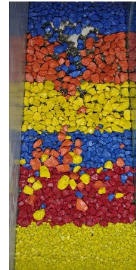
S_d = 4.6 Structure failed
