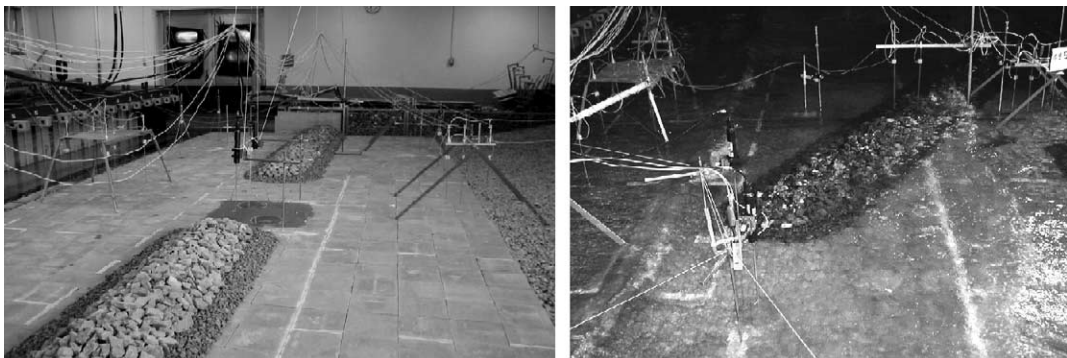
Fig. 8. Photo of set-up. Layout 1 at the left hand-side: two half round-head structures with a rip channel in between; Layout 2 at the right hand-side: a single breakwater inclined at 30° with respect to the beach.
