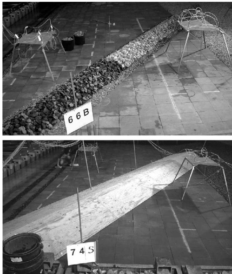
Fig. 12. Views of the basin, 30^\circ tests on rubble and smooth plywood structure.
