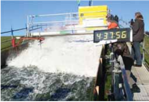
Figure 3. The Wave Overtopping Simulator releases 22 m 3 of water over 4 m width in about 5 s. It simulates a large overtopping wave with a mean discharge of 75 l/s per m.
