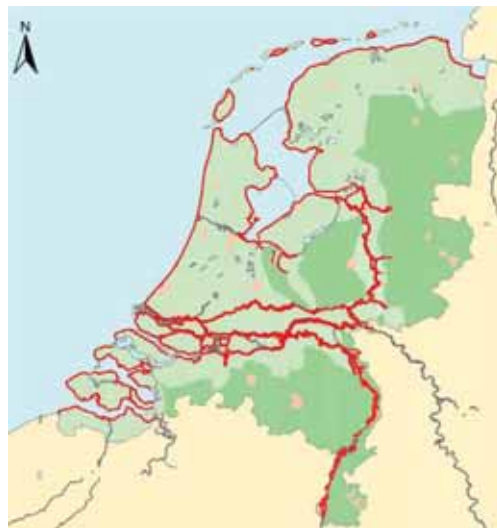
Figure 1. The Netherlands as delta with all primary flood defences, both for coastal and river protection.
