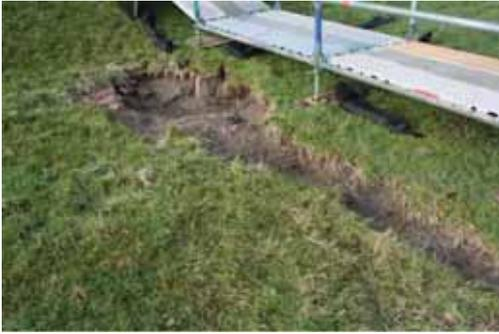
Figure 14. Result section 2 after 75 l/s per m.
