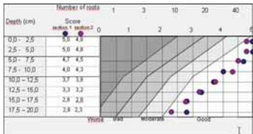
Figure 3. Root density February 2008, sections 1 and 2 (diagram VTV, 2006).
