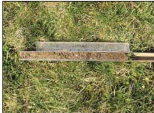
Figure 2. Gouge bit with 0.25 m sample of top layer.
