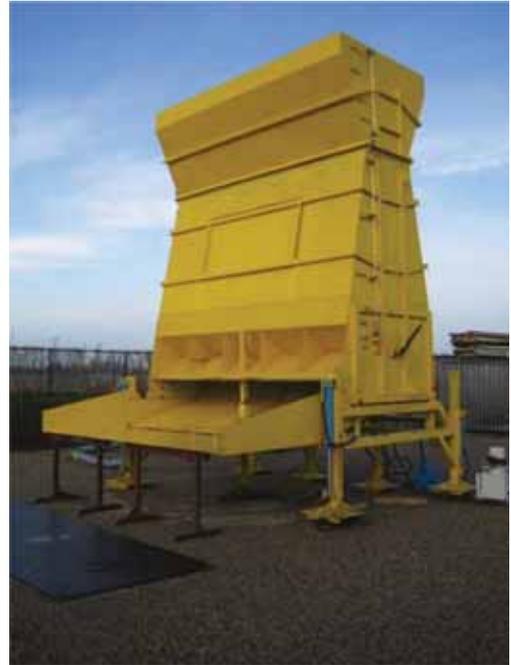
Figure 5. Enhanced wave overtopping simulator.
