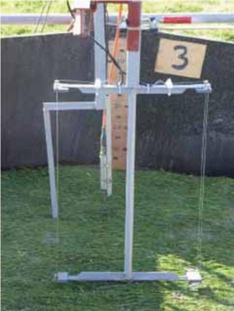
Figure 9. Flow depth instrument.
