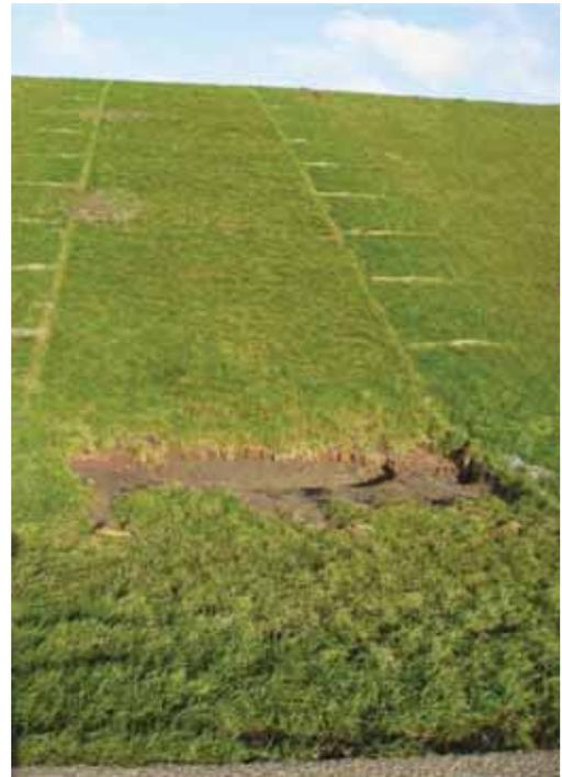
Figure 13. Damage test section 1 after 75 l/s per m.
