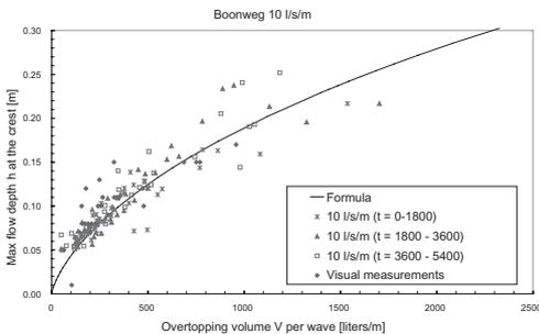
Figure 10. Flow depth measurements.
