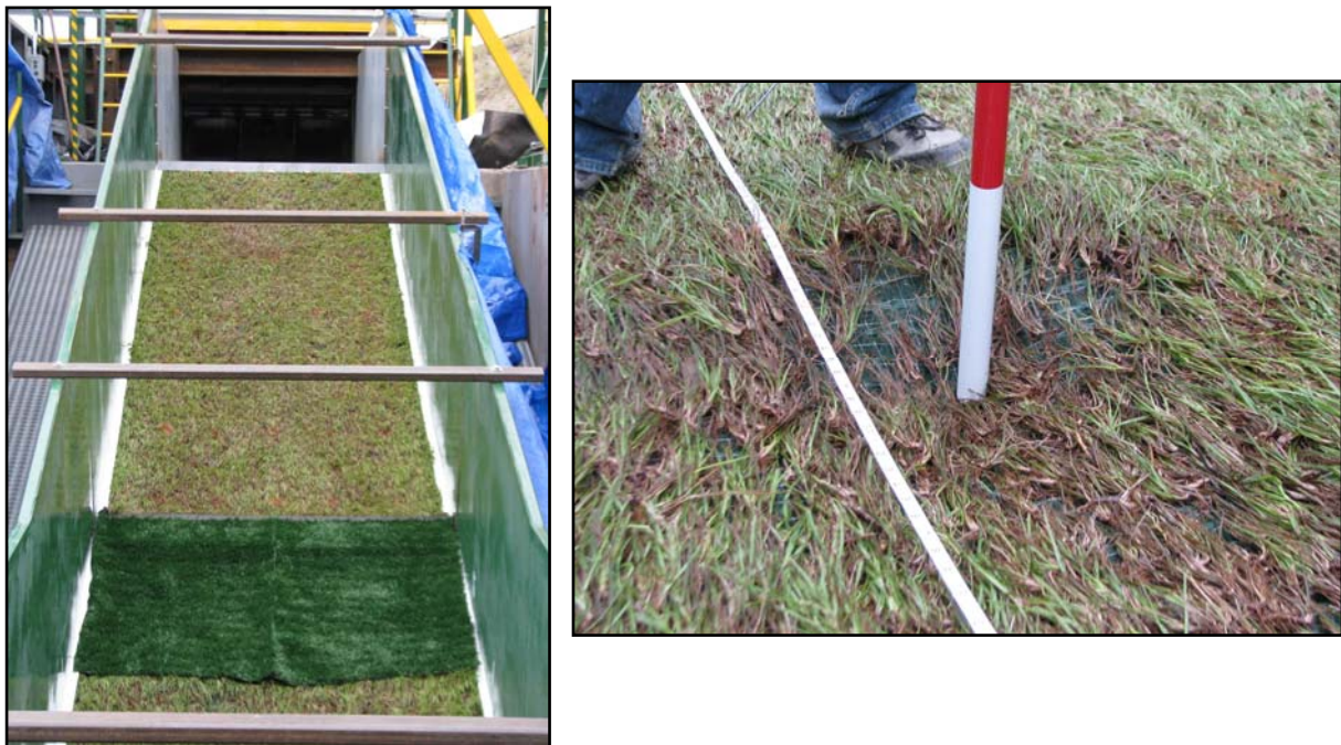
Figure 8. Grass reinforced with TRM (Test 6).
