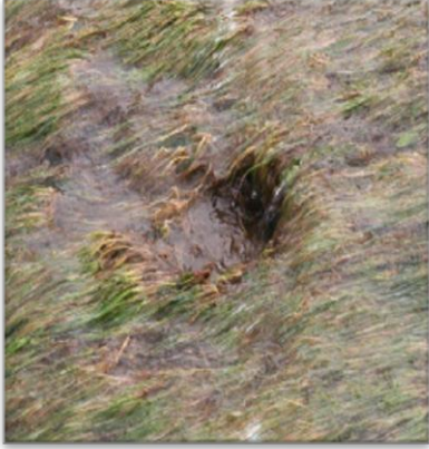
Initial damage ( D < 500 \text{ m}^2/\text{s}^2 )
