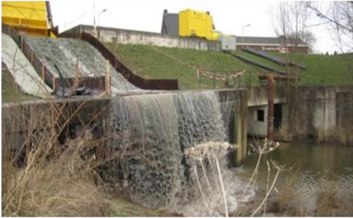
Figure 1. Tested transition: from grass to concrete.
