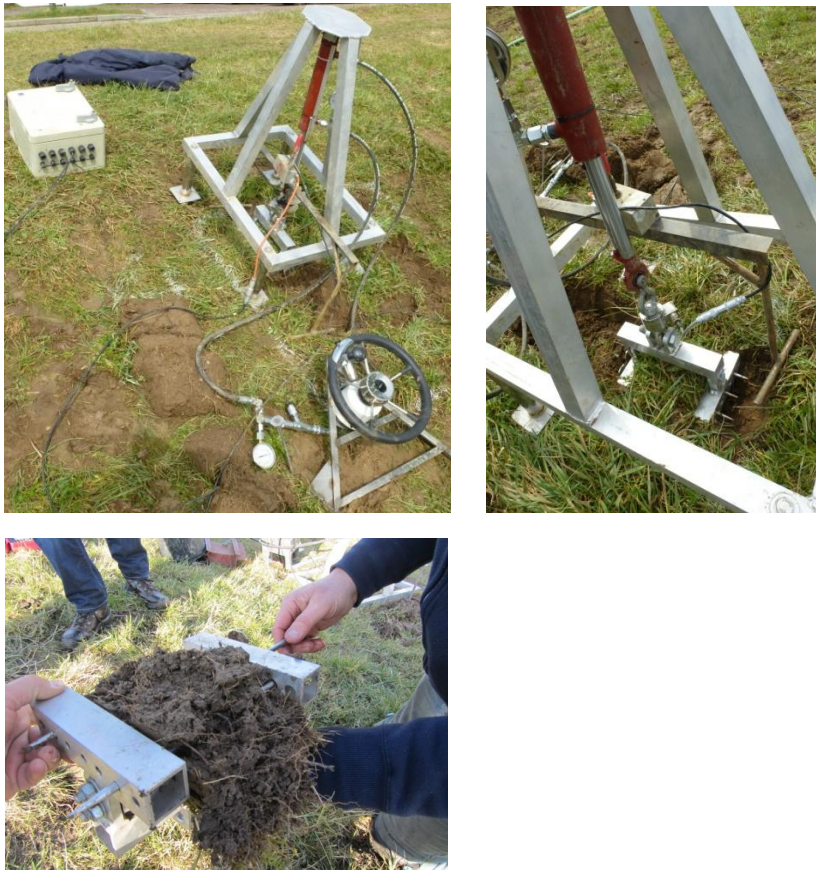
Figure 9. Grass pulling test device
