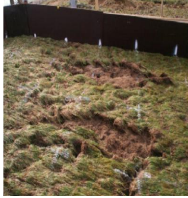
Damage at various locations or multiple open spots ( 500 \text{ m}^2/\text{s}^2 < D < 1500 \text{ m}^2/\text{s}^2 )
