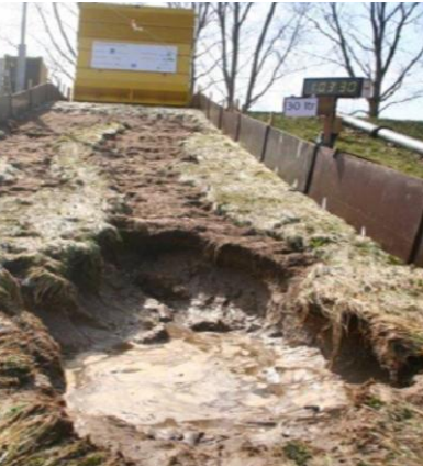
Failure ( D > 3500 \text{ m}^2/\text{s}^2 )
