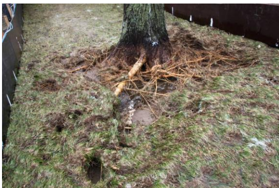
Figure 5. Erosion at tree (earlier test at Vecht dike);
