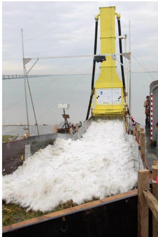
**Figure 5. The Wave Run-up Simulator in action.**
