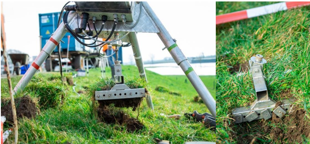
Figure 2. A GPT with the upgraded device (left picture). The pull frame is attached to the grass sod with steel pins (right).
