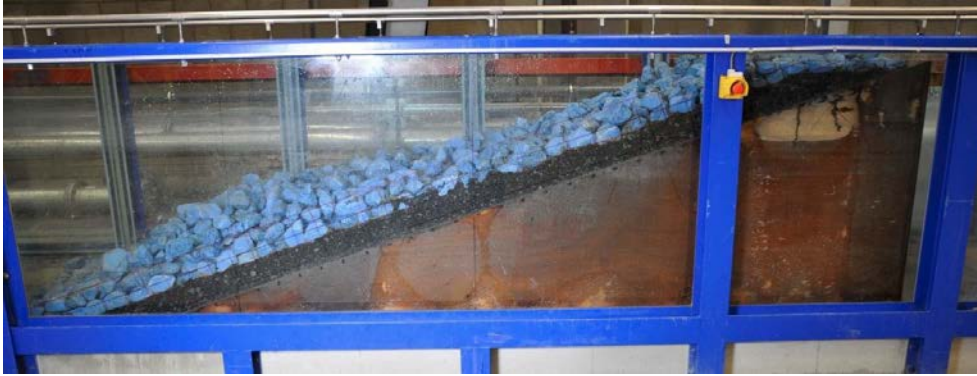
Figure 5: Picture of damage profile in the flume after finalising test 6 with the same, but thicker underlayer than in test 2, Figure 4. Note that S_d = 8.8 , about half the damage in test 2.
