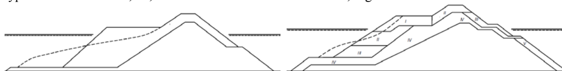
Figure 1. Mass armoured berm breakwater to the left, MA, and Icelandic-type berm breakwater to the right; IC. On both cross sections the expected reshaping is shown with a dotted line.
