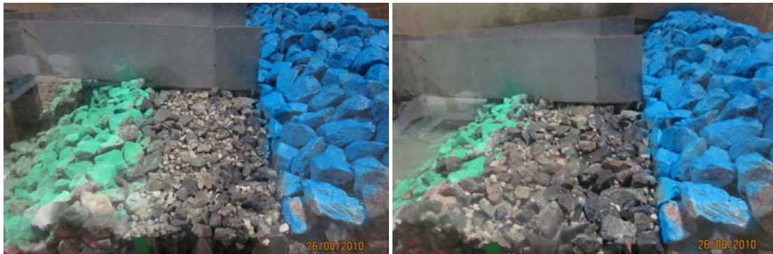
Figure 17. Model testing of an Icelandic-type berm breakwater similar to the Husavik berm breakwater, crest of blue stones to the right, unpaved road in the centre and rear side revetment on the left of both photos. The left and right photos are taken after wave conditions corresponding to stability numbers H_s/\Delta D_{n50} 1.4 and 1.6 respectively and with measured overtopping rate of 0.6 and 2.4 l/s/m respectively
